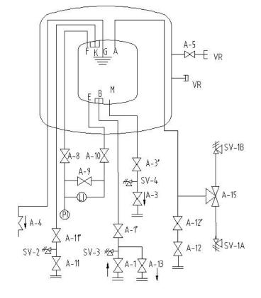
Vertical tank for liquid carbon dioxide
